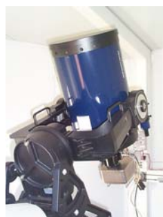
Left: Mt Kent Observatory's robotic telescope is a fork-mounted 30cm Meade LX200 Schmidt-Cassegrain telescope equipped with a CCD imaging camera and housed in a custom octagonal "dome". The robotic observing system comprises an interconnected network that includes the telescope, camera, dome and auxiliary electronics. Custom software controls operation of the system, including dynamic scheduling of observations according to external factors, especially on-site weather conditions. Right: The telescope's octagonal "dome" enclosure.
