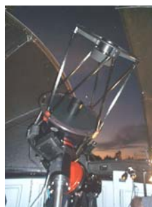
Left: The new Celestron-20 50cm astrograph at Mt Kent Observatory. The optics have a novel corrected Dall-Kirkham Cassegrain design with a 2-element corrector lens near the focal plane. Attached to the telescope is an SBIG STL-6303 2048 x 3072 format 9µm pixel CCD camera which gives a 18.64' x 27.96' flat field with 0.546" square pixels. Ray-tracing results and star tests indicate image quality with the corrected Dall-Kirkham design is superior to a Schmidt-Cassegrain design, and a wider flat field of view results that is better suited to CCD imaging with large-format detectors. The telescope's German equatorial mount also permits tracking objects up to 30° past the meridian before meridian flip of the mount is required. Right: The telescope is housed in a Sirius Observatories 3.5m diameter fibreglass dome.
